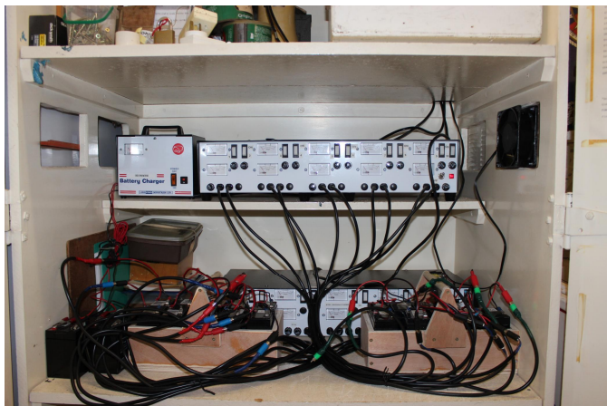
Above photo shows the two chargers in the Boat Cupboard with the two new battery boxes that hold ten batteries each. Much easier to carry than the previous single box of 18 batteries
